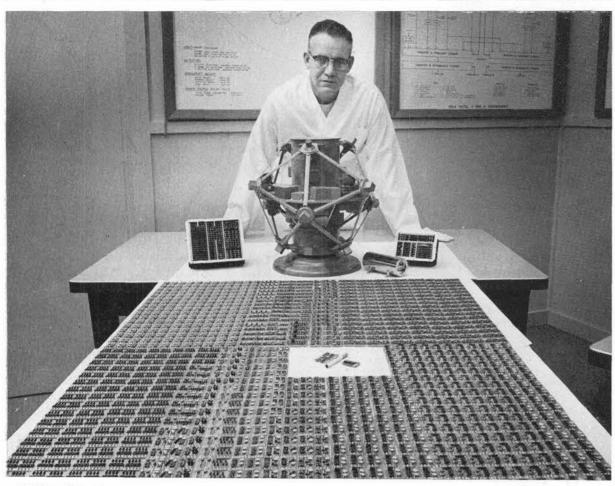
MULTITUDES of miniature components make up the Sandia Corporation-designed logics systems of the detector satellites. The modules are displayed by Robert D. House (7432-1), a member of the Sandia
